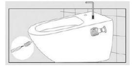
10. Once the installation is completed, a flush and leak test should be carried out and once it has been commissioned, the toilet can be sealed around the edge to finish.
