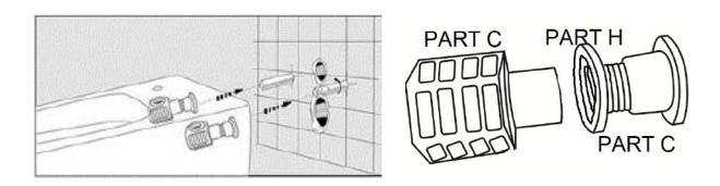
Please note: The cut out on the connector and the hole in the housing should be aligned.
